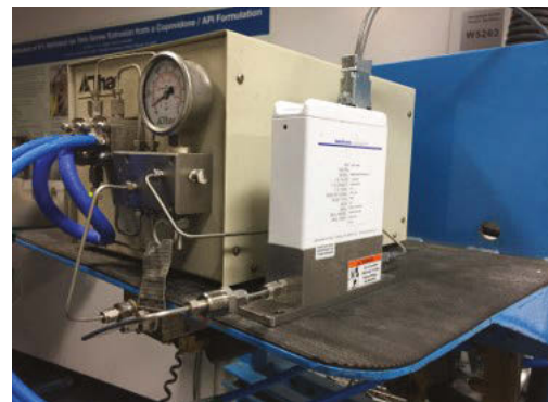
Piston Pump and Brooks Quantim Coriolis Flow Meter
