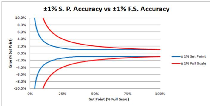
Figure 2: Plot comparing ±1% of set point accuracy to ±1% of full scale accuracy. Please note that for the set point accuracy it is ±1% of set point between 35-100% control range, and 0.35% of Full scale from 2-35% control range.
