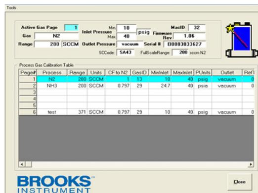
Figure 12: Saved gas configurations show up in the Process Gas Calibration Table
