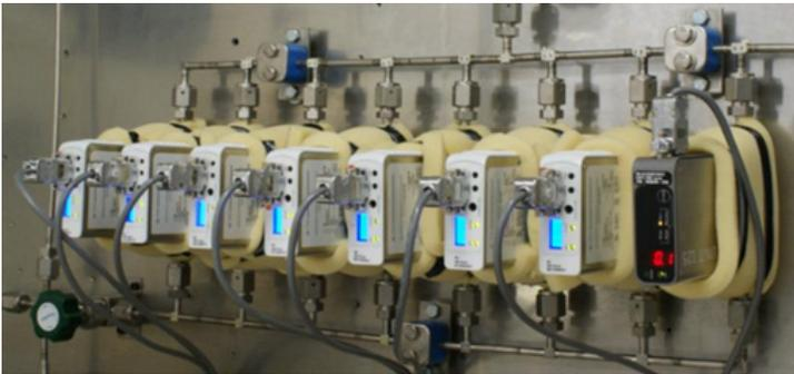
Figure 1: Data is collected in our state of the art Gas Lab on multiple MFCs in order to create an extremely accurate gas data base
