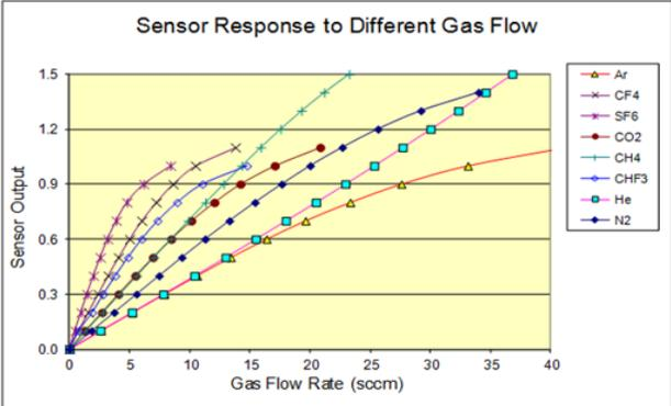
Figure 3: Flow sensors respond very differently with different gases. While gas conversion factors may work better for some gases, most do not have a linear relationship between the flow rate and the sensor output which causes inaccurate readings
