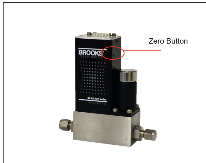
Figure 3-1 Externally Accessible Adjustment (Zero Button) for all Meters/Controllers.
