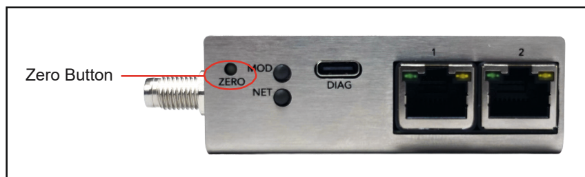
Figure 3-1 Externally Accessible Adjustment (Zero Button) for all Meters/Controllers.
