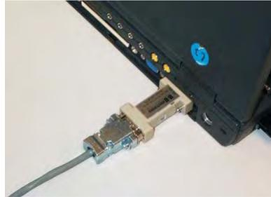
7. Connect the 3-wire communications cable to the device's service port, which is the black connector located behind the D-connector. Align the communications cable's 5-pin connector with the **black wire** towards the **center** of the device (towards the LEDs), as shown in the following illustration.
