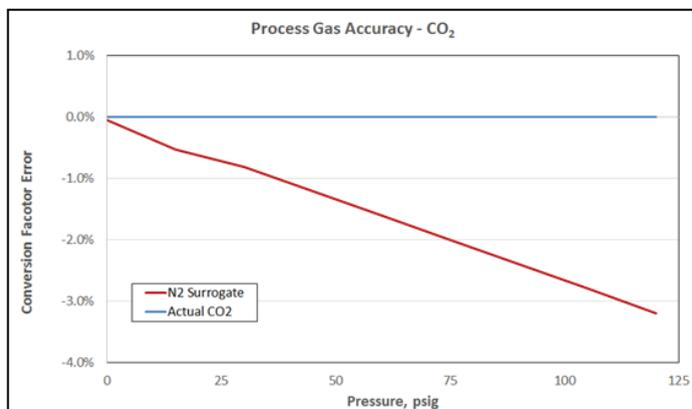
*CO<sub>2</sub> is a refrigerant, which makes its conversion factor highly pressure dependent; using N<sub>2</sub> as a surrogate calibration gas introduces inaccuracy in CO<sub>2</sub> delivery.*
